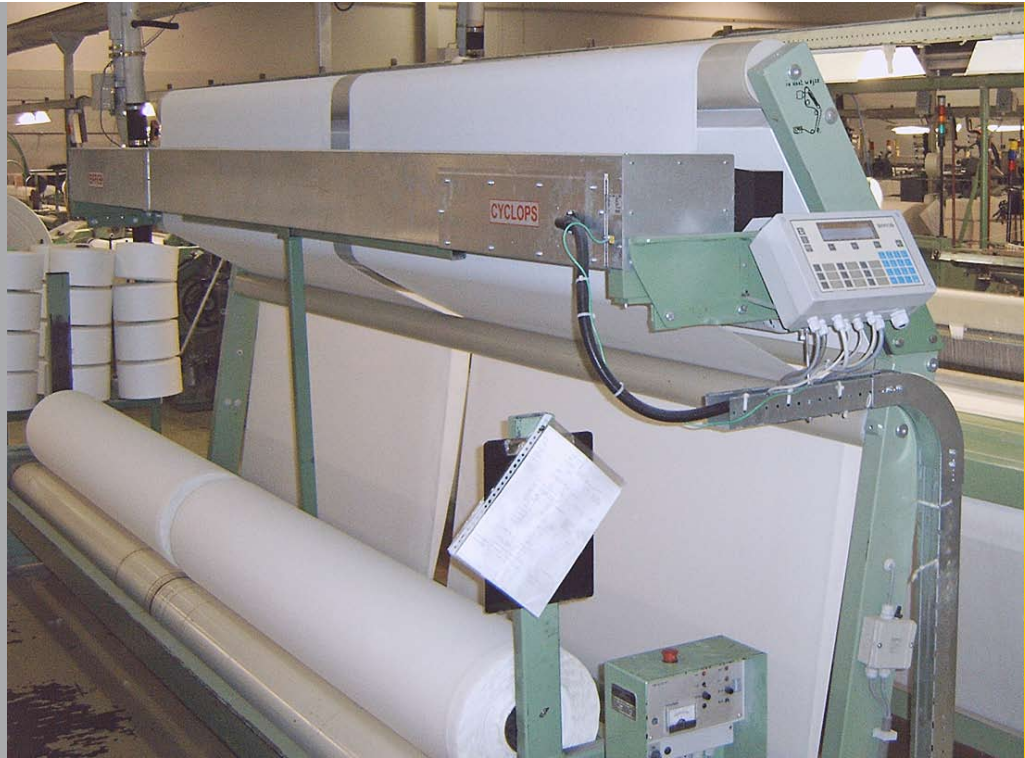
Fig. 1: Cyclops is mounted on the off-loom take up and uses one or two moving camera units scanning the fabric for possible defects. A data unit serves as interface between Cyclops and the loom.
