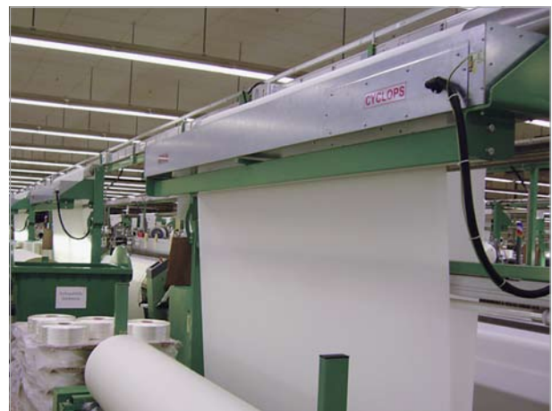
Fig. 4: Air jets weaving air bag fabric, equipped with Cyclops at UTT.
