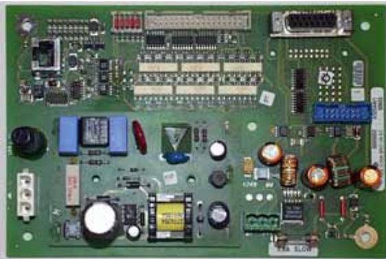
A5054401 - FF connection board 230VAC
