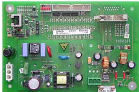
A5054403 - FF connection board 230VAC stand-alone
