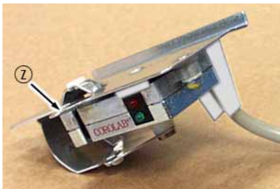
A905044 - Q-detector LU2 cylindrical
