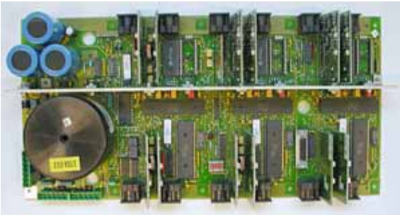
A569491 - Q-board LU2-E (with eprom) A5694915 - Q-board LU2-E-DL (with flash)
